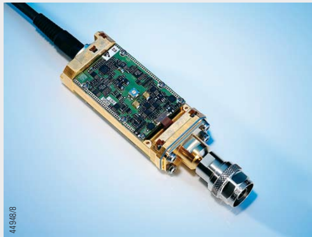
FIG 3 Compact, high-precision electronic design: internal circuitry of the R&S®NRP-Z81 wideband power sensor.
