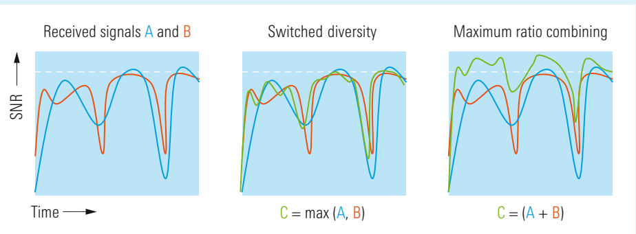
FIG 3 Comparison between switched diversity and maximum ratio combining at a receiver with two antennas.
